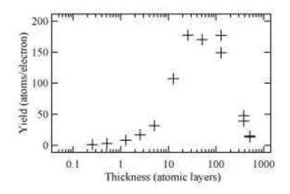
Fig.1 Total desorption yield of Ne by electron impact as a function of the thickness of Ne films. Electron incident energy is 120eV.
